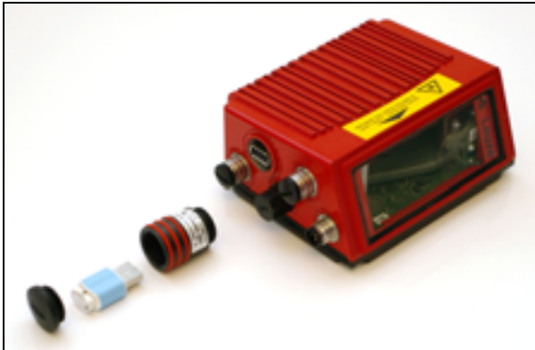
Figure 10.4: Installing the external parameter memory
