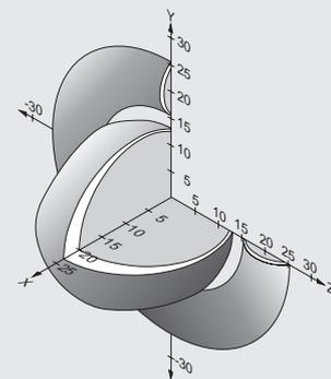
For a side approach direction for the actuator and safety switch, a minimum distance of  $s = 3$  mm must be maintained so that the operating distance of the side lobes is not entered.
