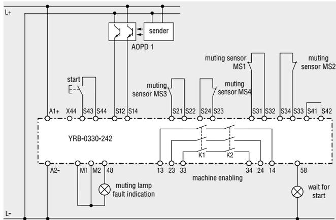
Diagram 3: Protective operation with muting via 4 muting-sensor contacts
