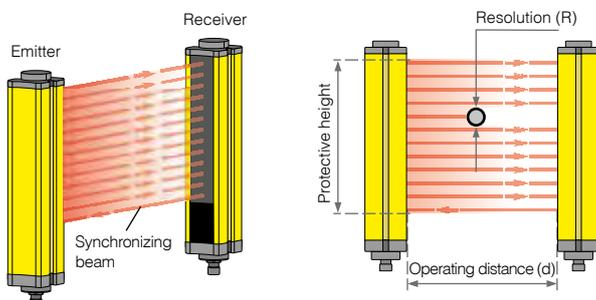
Reception of all beams activates the two independently generated semiconductor outputs (OSSDs) of the receiver unit. The interruption of one or more beams deactivates the outputs within the response time of the AOPD. Any internal fault is detected by the device's permanent self-control function and has the same result as an intrusion into the protective field.
