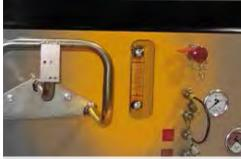
Application of HCX. column level indicator with incorporated thermometer.
