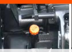
Application of SFP+a filler breather cap with splash guard and dipstick.
