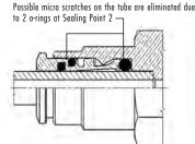
**Sealing point 1** is the traditional sealing point on a push-in fitting. While the additional **Sealing point 2** works on fresh tubing (non scratched), as well as keeping dirt and debris from entering tube gland and fitting
