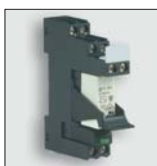
DC relay, 2 changeover contacts, pluggable, AgNi, AgNi +5 μm HV
