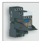
DC relay, 4 changeover contacts, pluggable, AgNi, AgNi +5 μm HV
