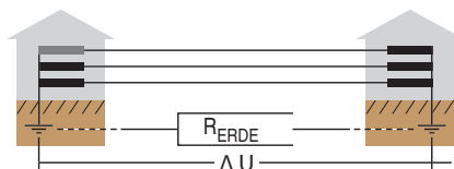
Potential differences due to earth loops
