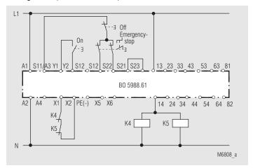
Contact reinformcement by external contactors with reduced safety level.
