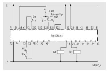
Contact reinforcement by external contactors, two-channel.
