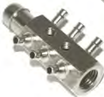
Special manifold, 1/8" female inlet, two 10-32 female outlets, six #3 barb outlets, and one #10 outlet; electroless nickel plated brass
