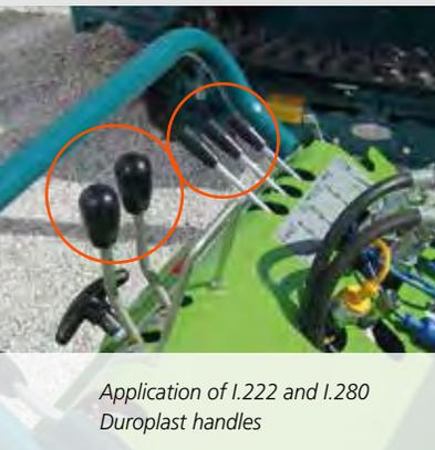
Application of I.222 and I.280 Duroplast handles
