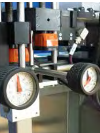
Application of MBT-GA knobs with integral gravity position indicator.
