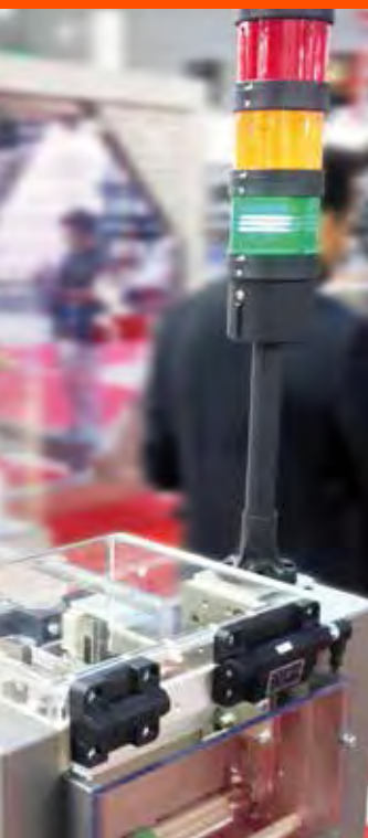
Application of CFSW. hinges with multiple safety switch.
