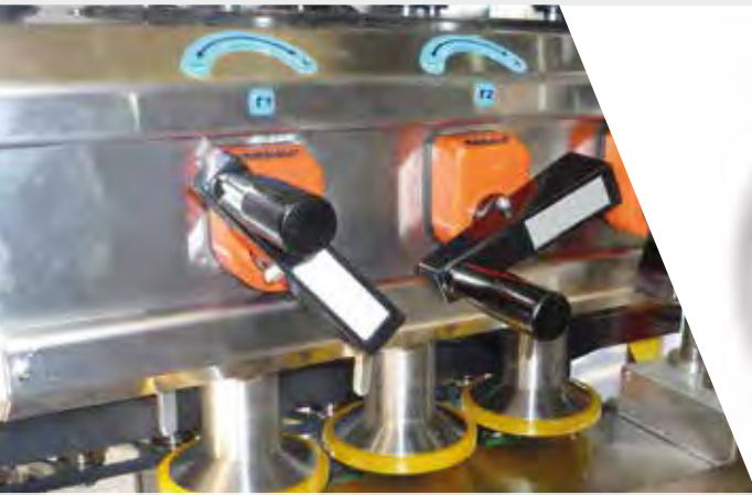
Application of DD52R direct drive digital position indicators and ME. balanced crank handles
