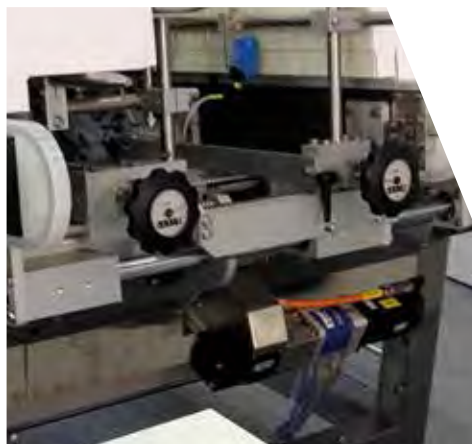
Application of VHT lobe knobs for position indicators and GW12 digital-analogue gravity position indicators.
