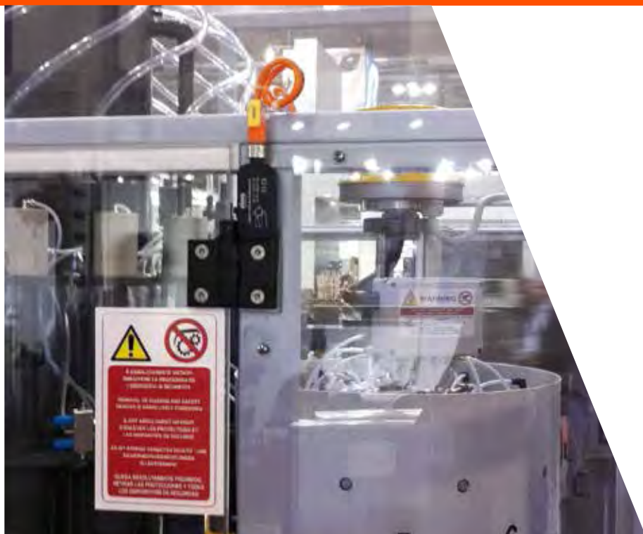
Application of CFSQ hinges with built-in safety switch.
